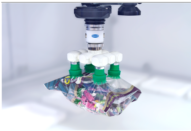
Bellows suction cups SPB4f when handling pouches
